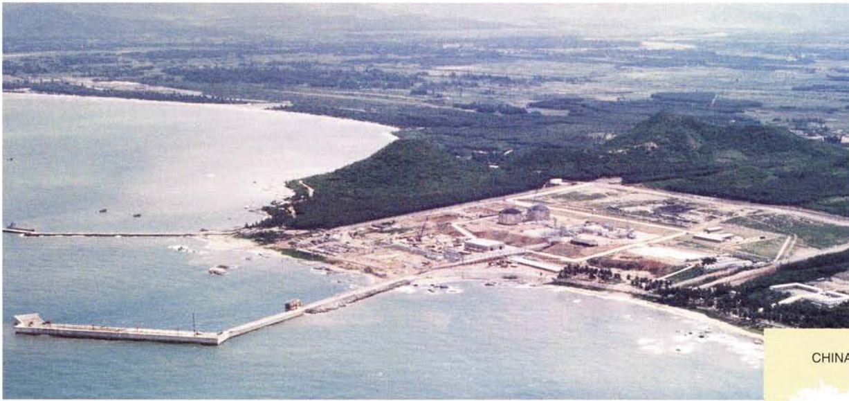
Output from the Yacheng field is piped to the Nanshan shore base (left) on Hainan Island. The field also supplies the Castle Peak Power Stations (below) in Hong Kong via a 770 km pipeline. (Photos: ARCO)
